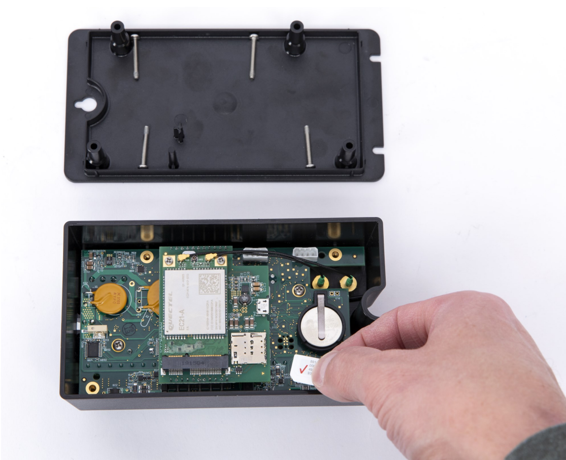
FIGURE 11-1. SIM card installation
